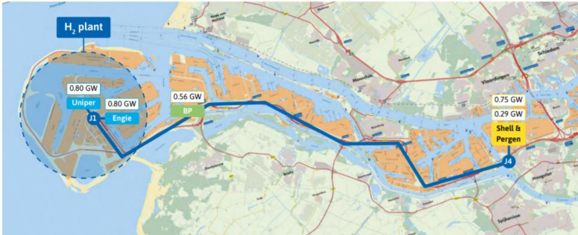
Figure 6.10: Reference scope case overview of the blue hydrogen production and transport infrastructure for the Rotterdam port, including both RFG and NG heating demand from end users. 'J#' are identifiers for junction points where the transmission pipeline splits into smaller lines going directly towards the plants.
